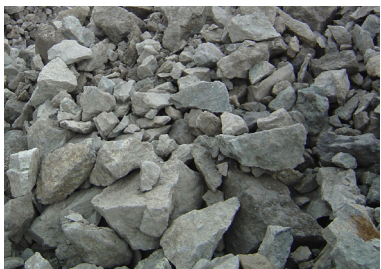
Feed material basalt 70 - 200 mm
