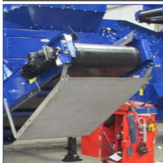
Magnetic Head Drum provides additional revenue by extracting ferrous metal from the waste stream
