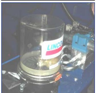
The auto-lube system provides reliable protection against friction and wear
