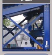
Air knife consisting of a 18.5KW motor. A lights cage is recommended along with this option
