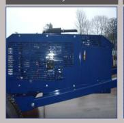
CAT2.2 Deisel/Hydraulic powerunit with a fuel consumption of 9.48ltr/ Hr (2.5USG)
