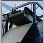
Head section over-band magnet with stainless steel chute to extract ferrous metal
